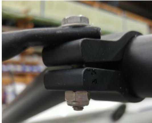
The backstay connects to the boat at the stern end of the footwell. It is held in place by a bolt that goes through the shell of the boat. With the rigger arm already secured to the boat, you must push this bolt back until it is flush with the hull of the boat for the backstay to line up properly. The picture below shows what this should look like.
