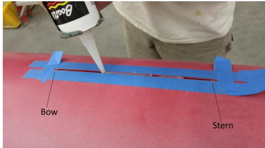
The fin slot is watertight even without the caulk, so there is no reason to use too much. The amount of caulk applied in the picture is about the maximum amount of caulk that you should apply. You want to avoid forcing caulk into the undercuts at the ends of the slot. Getting caulk in the bow undercut is especially undesirable because this will make removing the fin very difficult.
