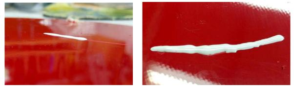
Note: the gel coat in your kit will be the same color as your boat. A contrasting color was used here to make the overfill more apparent.
