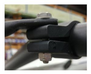
The backstay connects to the boat at the stern end of the footwell. It is held in place by a bolt that goes through the shell of the boat. With the rigger arm already secured to the boat, you must push this bolt back until it is flush with the hull of the boat for the backstay to line up properly. The picture below to shows what this should look like.
