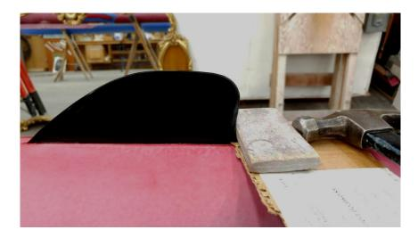
To force the fin towards the bow, you must hit it from the stern. The stern end of the fin is a small target and is fairly sharp, so use a block of wood to deliver the blows to the fin. The fin may be sharp enough to cut through the wood, so place it with the grain perpendicular to the fin. It is also recommended that you place a piece of cardboard underneath the block of wood to prevent damage to the hull.
