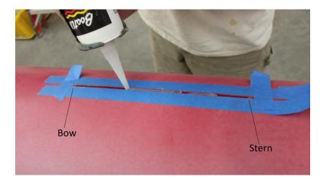
The fin slot is watertight even without the caulk, so there is no reason to use too much. The amount of caulk applied in the picture is about the maximum amount of caulk that you should apply. You want to avoid forcing caulk into the undercuts at the ends of the slot. Getting caulk in the bow undercut is especially undesirable because this will make removing the fin very difficult.
